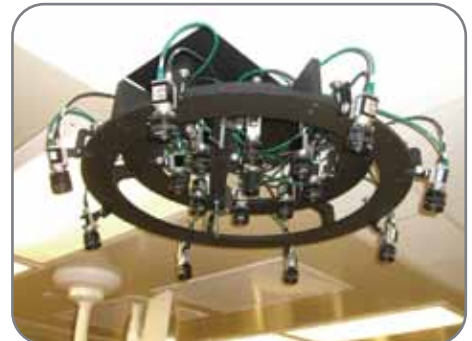
A camera array in operating theatre enables remote viewers to select different views of the procedure they are observing.
