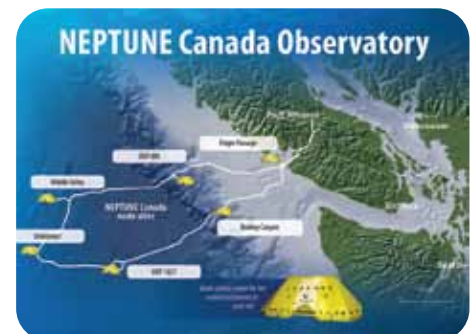
This map shows the distribution of NEPTUNE test nodes along Canada's west coast. The shallowest node is 50-100 metres deep, and the deepest is at 2.5 kilometres below the surface.
